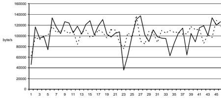
**Figure 1: Measured bandwidth (continuous line) and predicted bandwidth (dotted line) in a forty seconds time window.**
