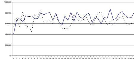
**Figure 2: Measured bandwidth with  $max_d = 6$  (continuous line) and with  $max_d = 2$  (dotted line).**
